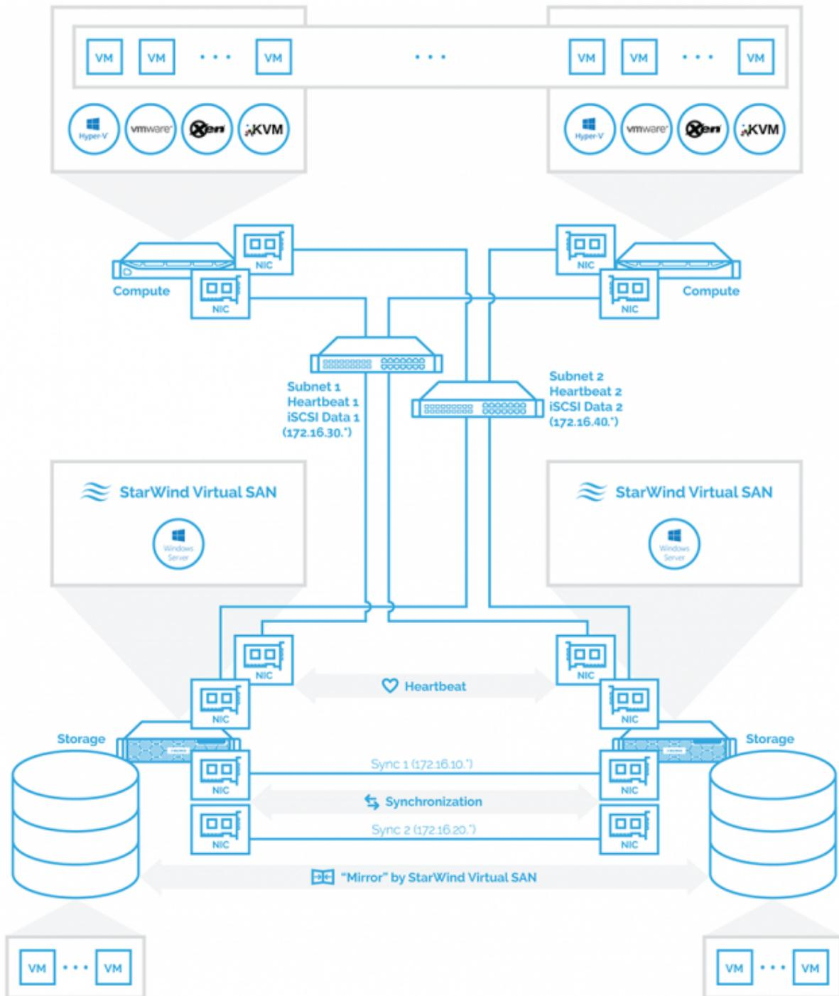
*Diagram 2: Compute and Storage Separated scenario setup.
