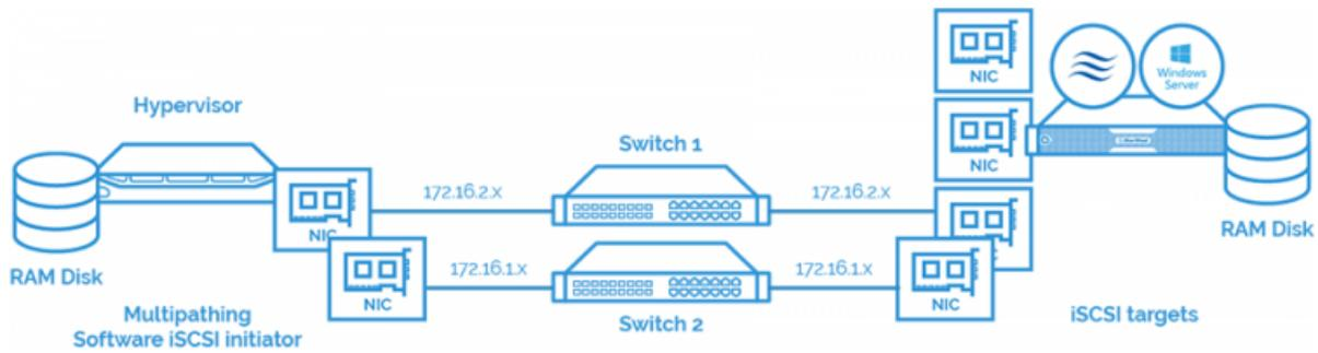
Diagram 4: RAM Disk connected via two paths.
