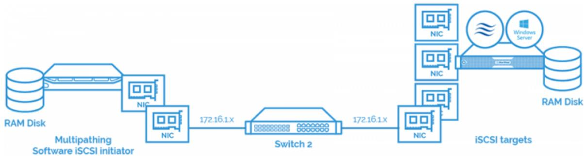
Diagram 3: RAM Disk connected via a single path.
