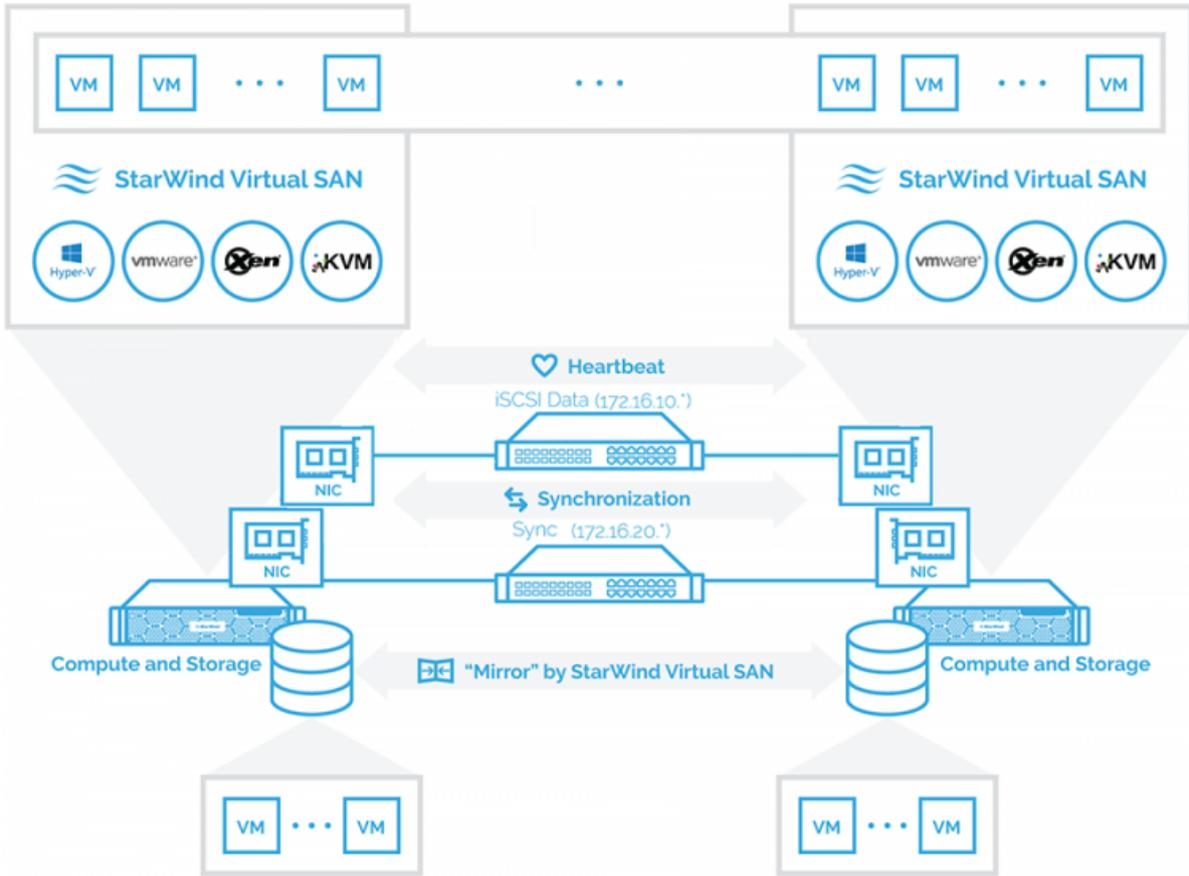
*Diagram 1: Hyperconverged scenario setup. Configuration: a two-node hypervisor cluster converged with StarWind Virtual SAN.*
