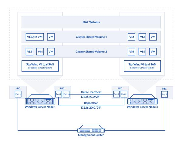
2-node StarWind HyperConverged Appliance with Hyper-V configuration diagram
