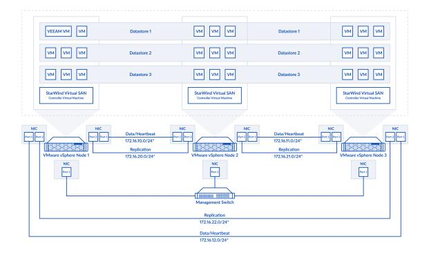
3-node StarWind HyperConverged Appliance (HCA) on VMware ESXi configuration diagram.
