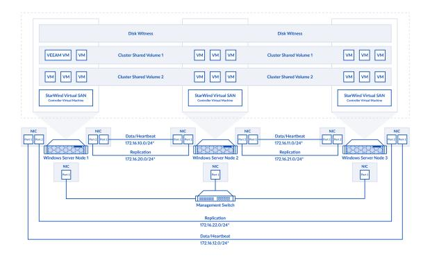
3-node StarWind HyperConverged Appliance with Hyper-V configuration diagram
