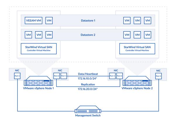
2-node StarWind HyperConverged Appliance (HCA) on VMware ESXi configuration diagram.
